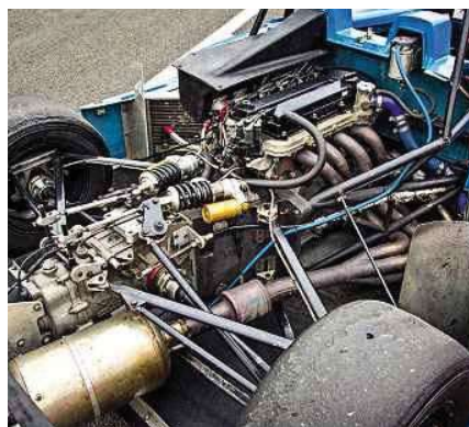
Left and above Modern Ford Duratec engine in place of the Pinto in older Sports 2000 cars; still glassfibre bodywork but F1-style suspension.
